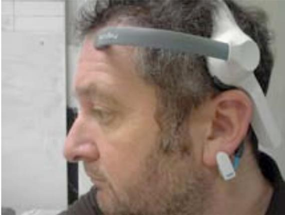
The Mindwave headset consists of the headset itself and a Bluetooth dongle. The headset will only work with the dongle and not any other Bluetooth device on the computer. It is important that these are removed or disabled as it can interfere with the setup.
